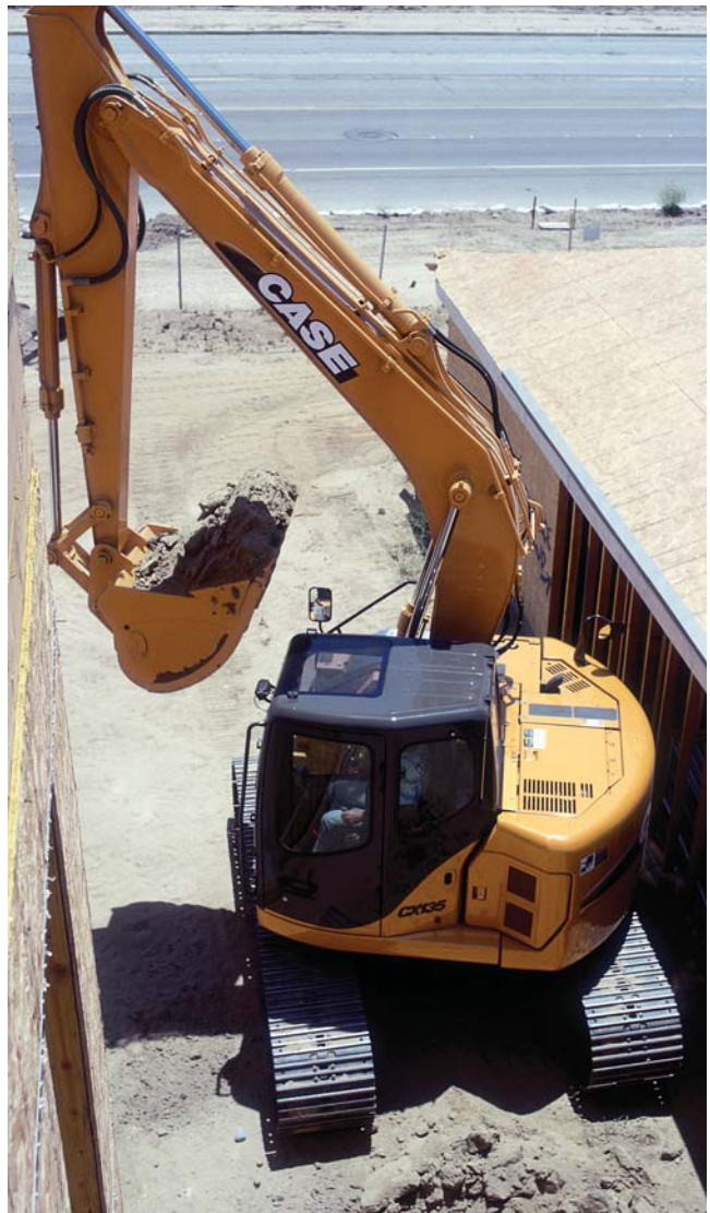
Configurations such as an offset boom, minimum-swing radius and zero-tail-swing allow excavators of all different sizes to work in tight quarters, such as residential backyards or crowded city streets.
