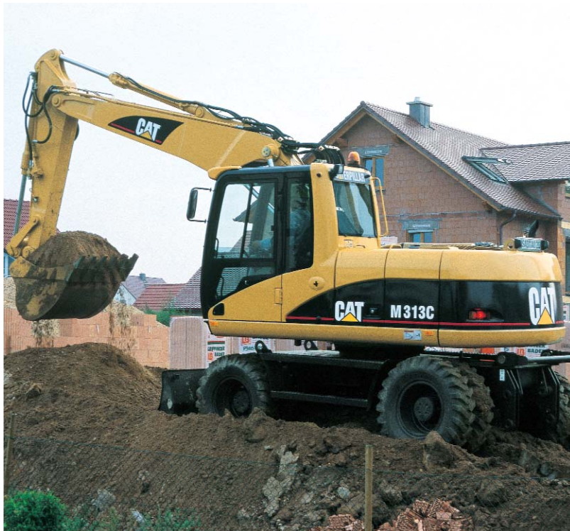
Tracked excavators are much more common than wheeled units, but wheels can be very effective when you need a little extra mobility on the job.
