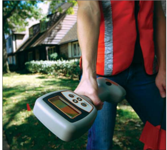
Simple units are a basic wand or box, while more sophisticated units are a wand with a larger display that can show more information and a larger antenna area.
